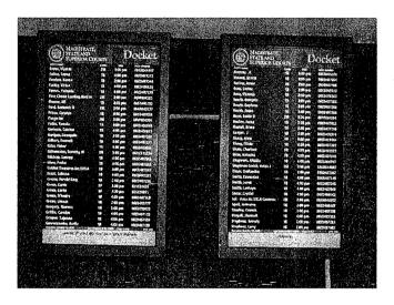
Reader board system hardware is fairly basic: the monitors, mounting hardware, a CPU (or two) with video card(s) for each of the monitors, and a data connection from the computer(s) to the network. The monitors are typically 32-inch to 50-inch LCD<sup>†</sup> flat screens. Depending on the location, the monitors may need to be placed within an enclosure to prevent damage.
